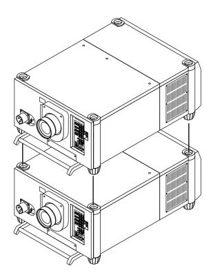
**CAUTION:** To prevent the projectors from falling, install them in a place and fasten them in a way with sufficient strength to support the two projectors.
